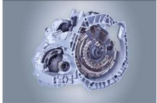
The 6DCT250 six-speed transmission has been designed for front-transverse installation in the mid-sized and compact vehicle segment for torques up to a maximum of 280 Nm. It can be equipped with a separate PTU with an all-wheel drive system, as well as a start/stop function without modification of the hardware. Combined with an electric motor, the transmission can also be used in a hybrid drive.
